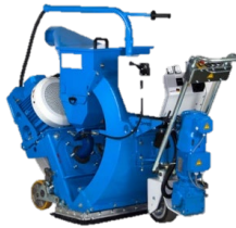
Fig.2: Grit blasting machine
